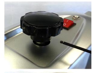
Loosen set screw in shaft of pressure adjustment knob and remove knob
