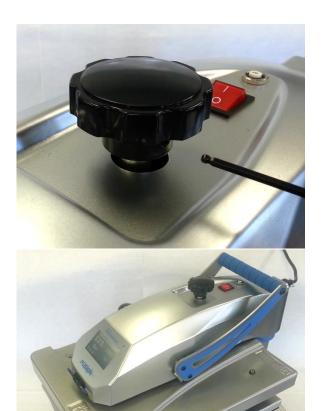
Replace Pressure Adjustment Knob, aligning set screw with flat of shaft and tightening with 3/32" Allen Wrench
